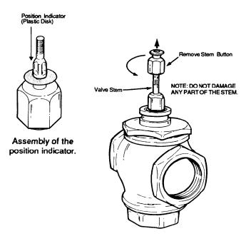
FIG.3 -- PREPARATION FOR VALVE ASSEMBLY.
